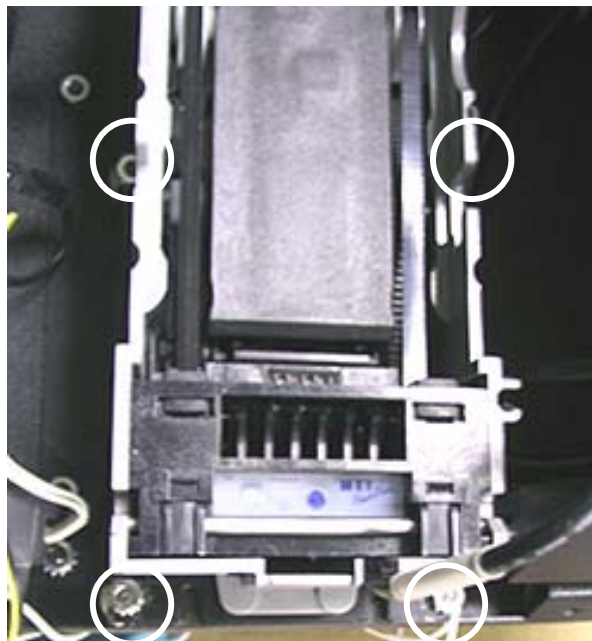
FIGURE 4 - SCREWS SECURING BILLACCEPTOR TO MOUNTING PLATE
