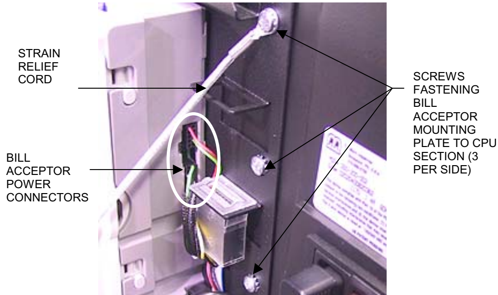
FIGURE 2 - REAR VIEW OF BILL ACCEPTOR MOUNTING PLATE
