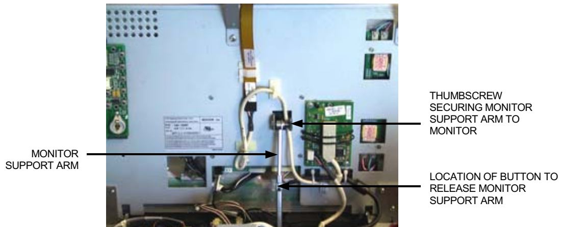
FIGURE 2 - REAR VIEW OF MONITOR ASSEMBLY
