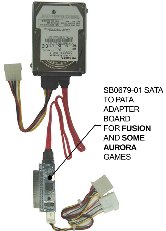
FIGURE 6 - NEW SATA HARD DRIVE ASSEMBLY FOR FUSION GAMES WITH ECS MOTHERBOARDS AND FUSION & AURORA GAMES RUNNING 2009 SOFTWARE OR EARLIER (SEE FIGURES 9 & 11 FOR DETAIL)
