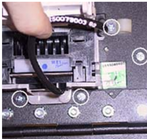
FIGURE 3 - SCREWS FASTENING SMALL BILL ACCEPTOR NOSE TO MOUNTING PLATE
