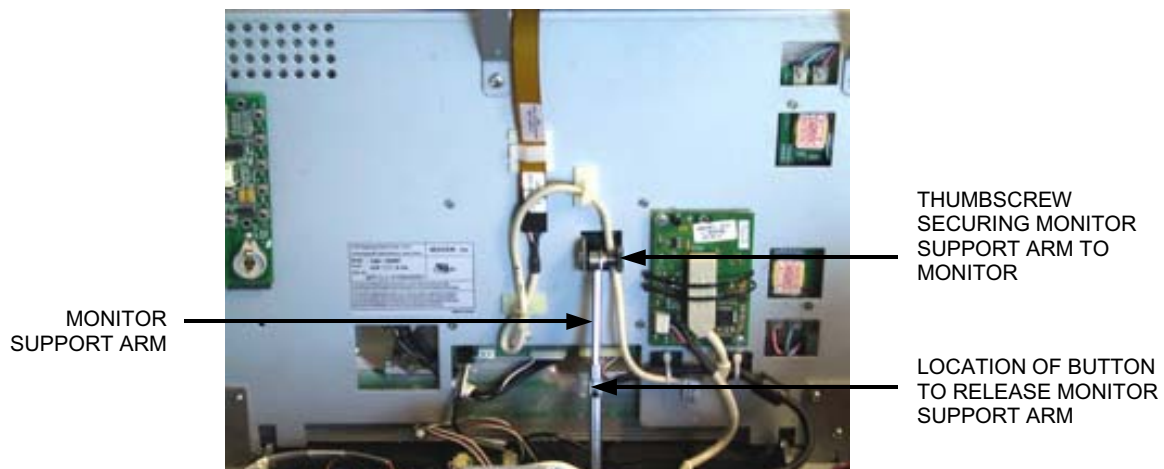
FIGURE 2 - SUPPORT ARM CONNECTION TO MONITOR
