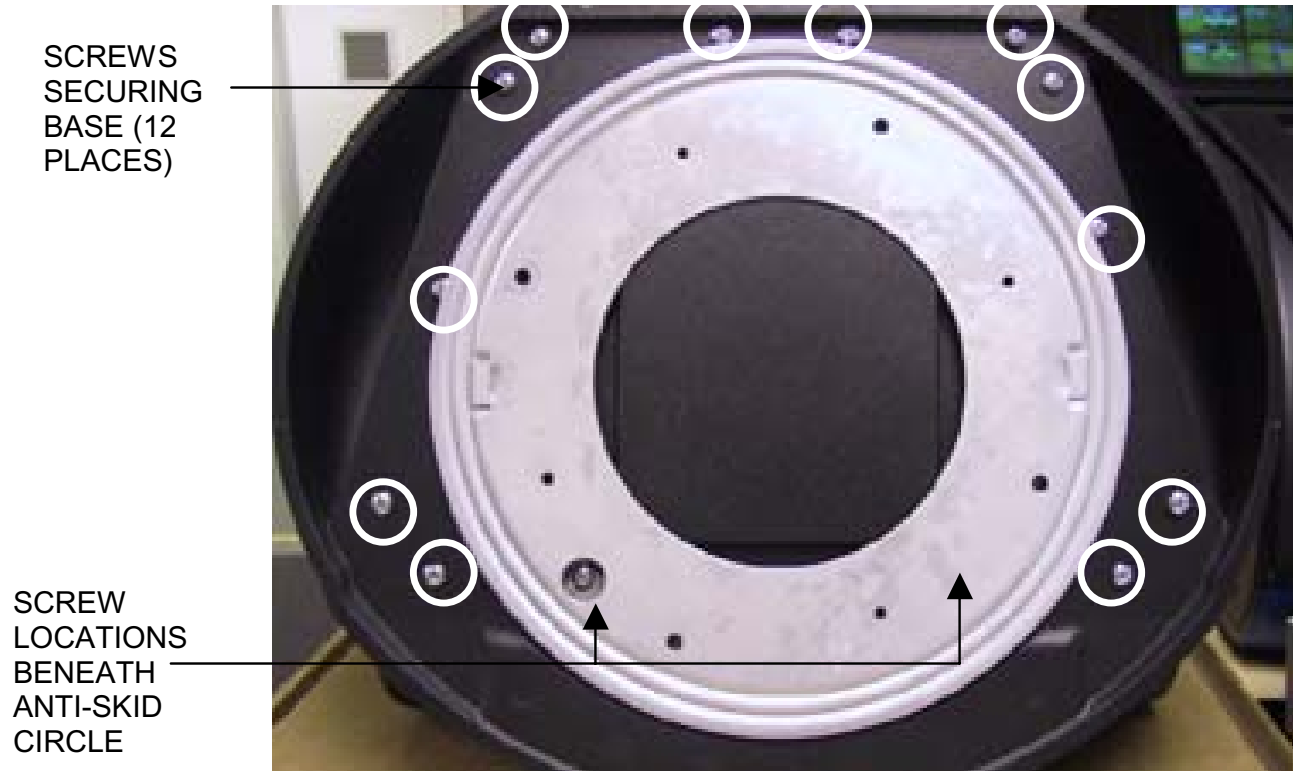
FIGURE 2 - ELITE EDGE - BASE AND ANTI-SKID CIRCLE REMOVAL
